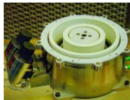
Engineering model of the ROS-2000 Hall-effect thruster (courtesy of Astrium)
