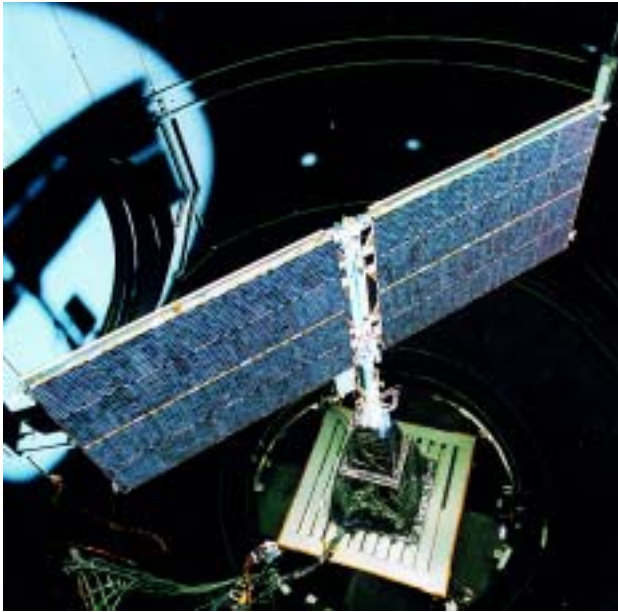
Flight model of the Hubble Space Telescope's solar array no. 3 in the Large Space Simulator (LSS) at ESTEC in Noordwijk (NL) in October
