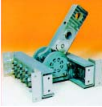
Ceramic-matrix-composite body-flap bearing assembly for the X-38 vehicle
