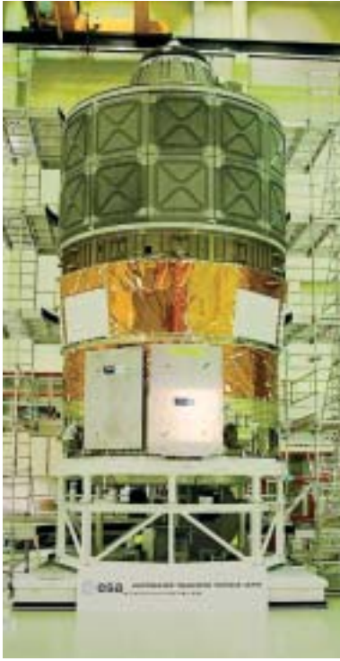
The Automated Transfer Vehicle (ATV) structural and thermal model at ESTEC (NL)
