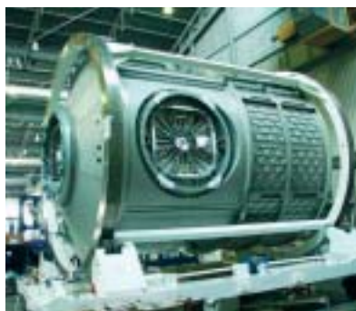
The Node-2 primary structure
