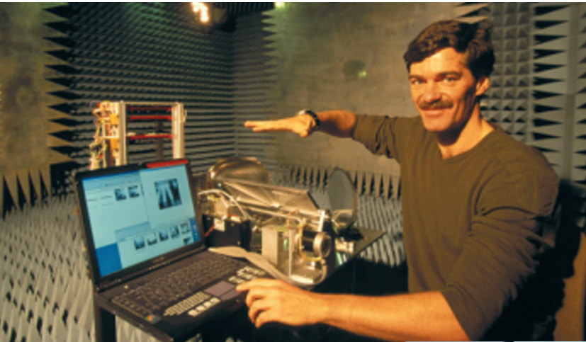
The advanced imager in operation, with the terahertz image of the hand captured on the laptop's screen
