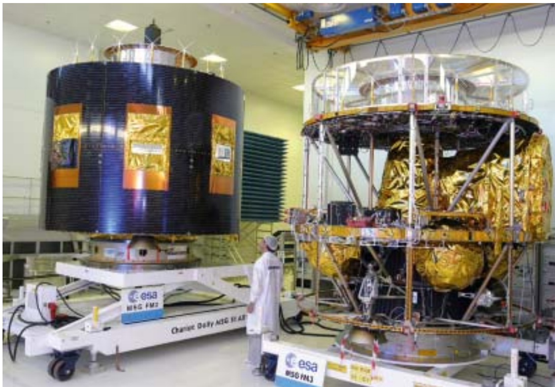
MSG-2 in flight configuration and MSG-3 in pre-integrated form in Alcatel Space's clean room in Cannes (F) (Courtesy of Alcatel Space)
