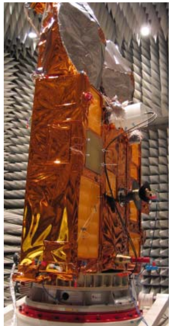
Flight model of CryoSat at IABG (D) for environmental testing
