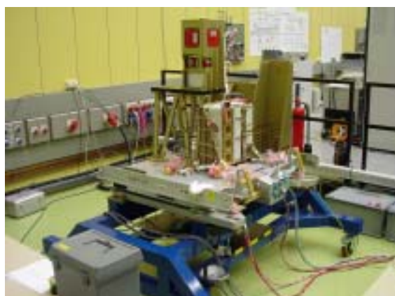
Interface testing of the first three experiments to be integrated on the EuTEF flight model
