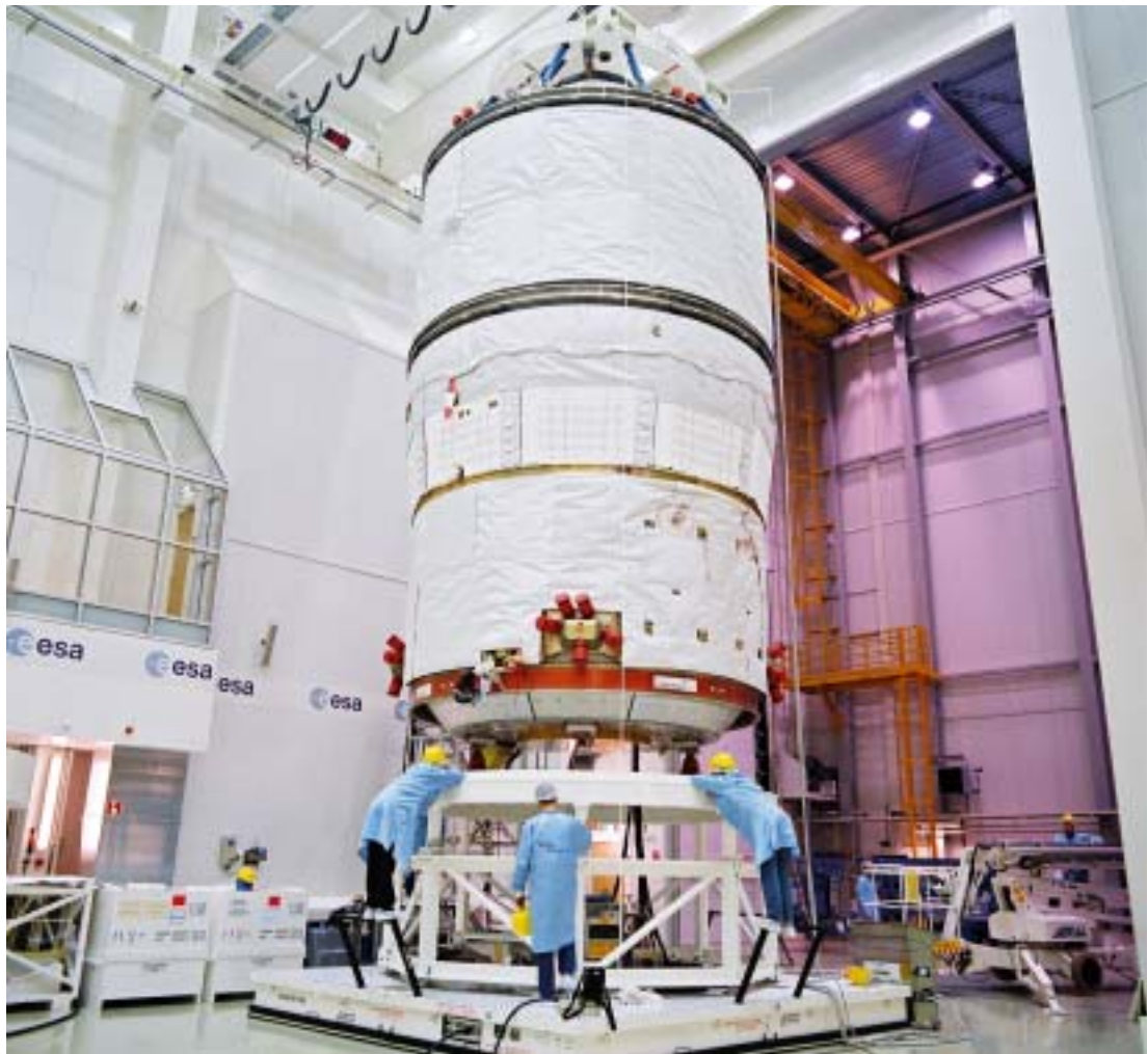
The flight model of the first Automated Transfer Vehicle (ATV-1) being prepared for environmental testing in the ESTEC Test Facilities
