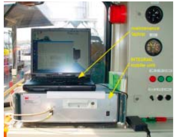
A prototype EGNOS-based train-locating unit, which forms part of a system known as INTEGRAIL, installed in a locomotive for test purposes (Courtesy of Bombardier GmbH)
