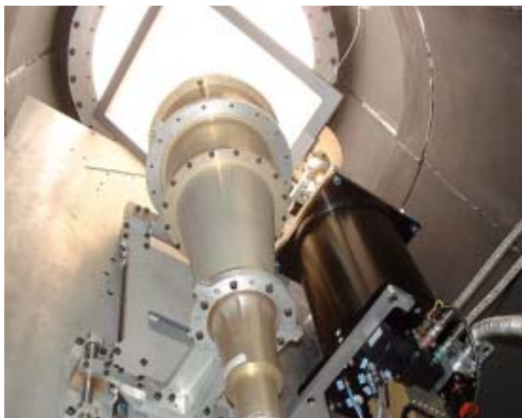
The new experimental Ka-band antenna system at the Villafranca ground station
