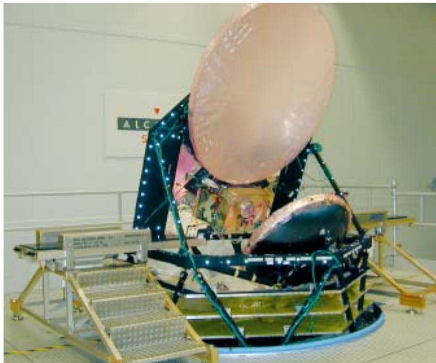
The qualification model of the Planck payload module, with its primary and secondary reflectors, at Alcatel Space in Cannes (F) prior to acoustic testing
