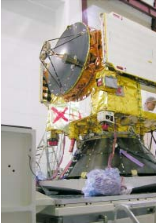
The Venus Express spacecraft in launch configuration for vibration testing at Intespace in Toulouse (F)
