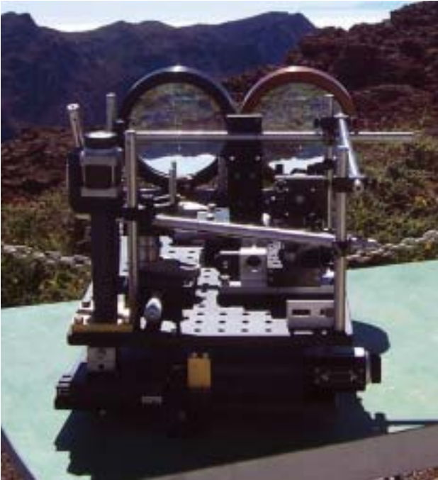
Photonic receiver aligned for encryption-key exchange between the Canary Islands of Tenerife and La Palma
