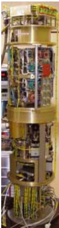
The Electromagnetic Levitation Module, flown for the first time on the Texus-42 sounding-rocket flight
