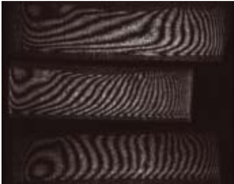
Interfacial turbulence in evaporating liquids (from the ITEL experiment on Maser-10)
