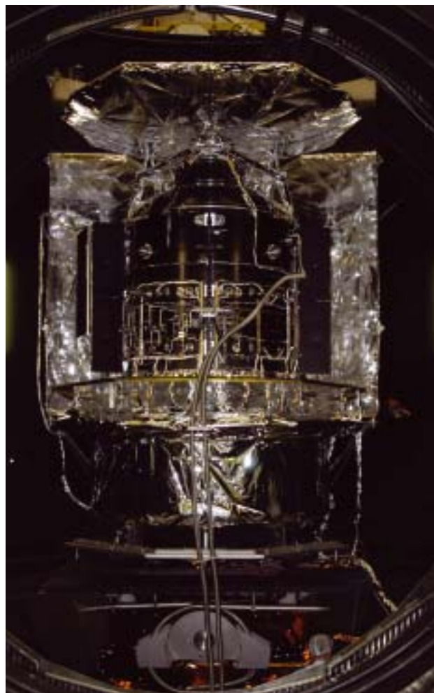
The Herschel structural and thermal qualification model spacecraft
