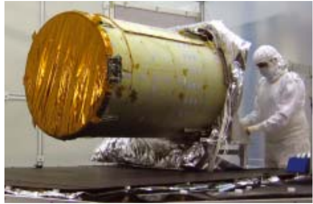
Integration of the baffle and deployable cover on the COROT flight model (Courtesy of CSL)
