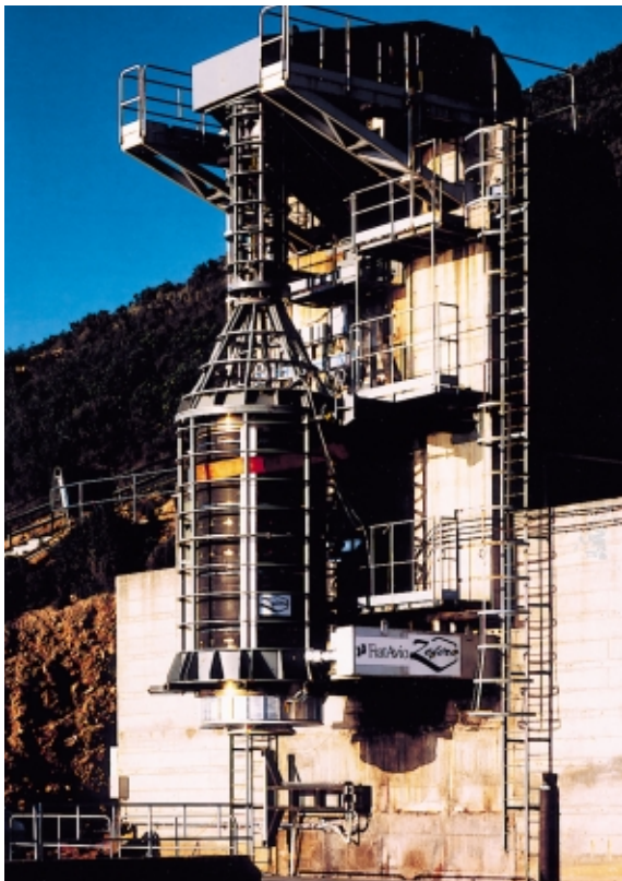
Test firing of Vega's Zefiro second-stage motor by FiatAvio, on 18 June
