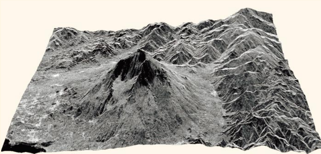
An ERS SAR image overlaid on an ERS-SAR-derived DTM of the Mount Etna volcano, Italy
