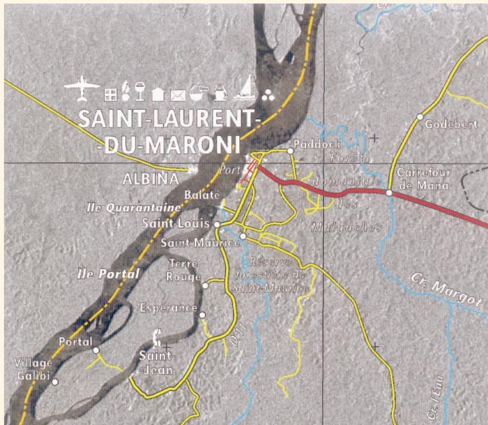
Example of a remote-sensing cartographic product derived from the mosaic. Marginal information, such as contour lines derived from the DTM, toponyms selected on the 1:200 000 map series and roads from the 1:50 000 map series, has also been integrated into the map. This does not bear the hydrographic network reference, as the main river channels can be easily detected. Here, the contribution of SAR is evident: land cover and topographic relief information can be extracted; forest areas, clearings, agricultural fields and settlements can all be identified
