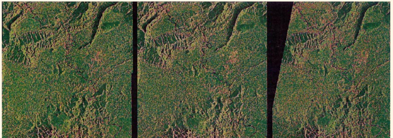
Demonstration change map for the Mahakam River region produced from three images (shown above) acquired on 12 July 1993, 29 November 1993 and 15 September 1994
