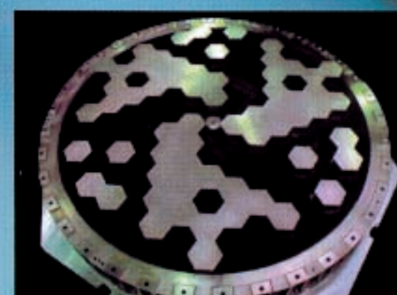
The coded mask being used on SPI. Photo: ESA
