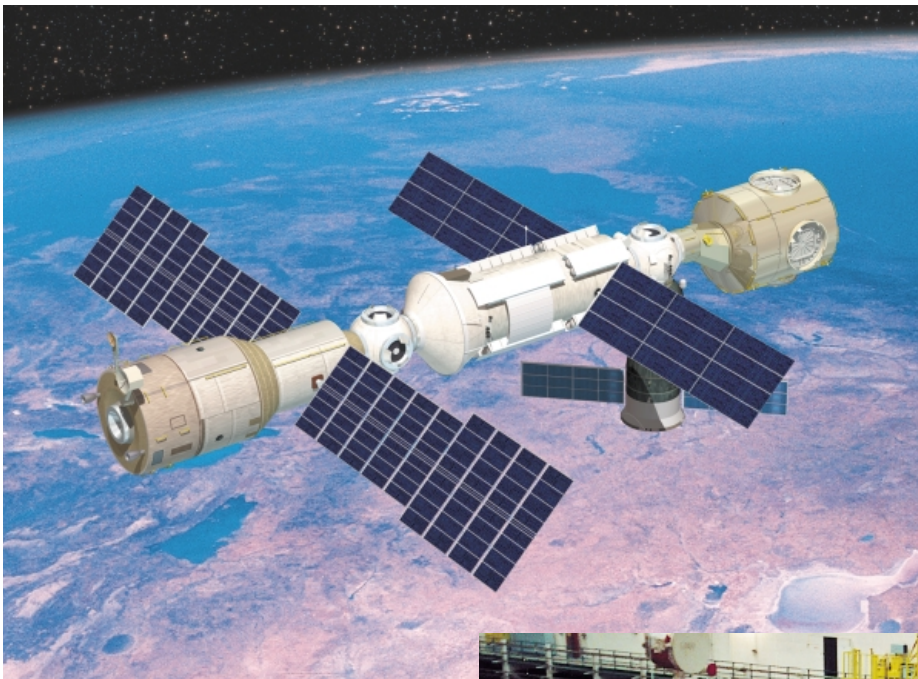
Zvezda (left-most module) is the third infrastructure element of the International Space Station (ESA/D. Ducros)
