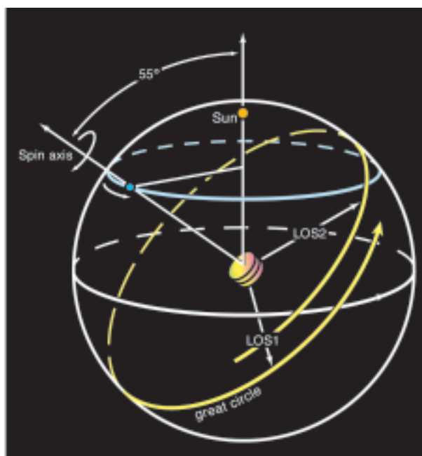
Figure 4. Characteristics of the observing strategy. The satellite rotates slowly about its spin axis, which itself precesses at a fixed angle of 55 deg to the Sun. LOS 1 and LOS 2 indicate the lines of sight for the two viewing angles which scan the same great circle on the sky
