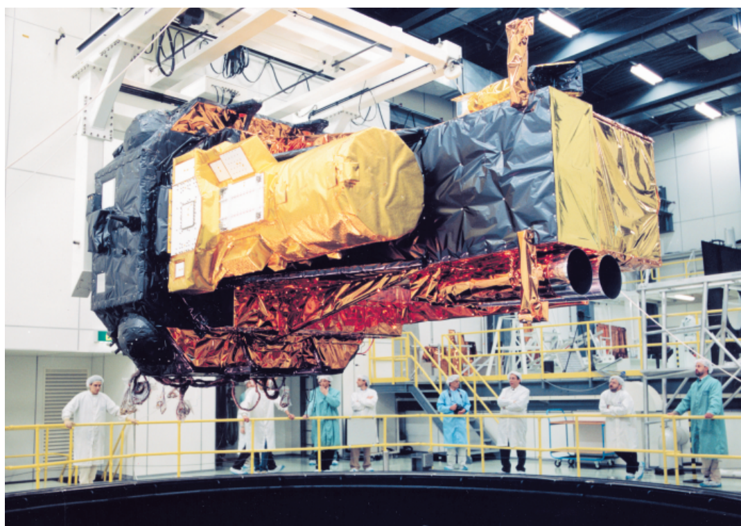
Figure 1. The Integral Structural Thermal Model being readied for testing in the Large Space Simulator (LSS) at ESTEC in Noordwijk (NL)
