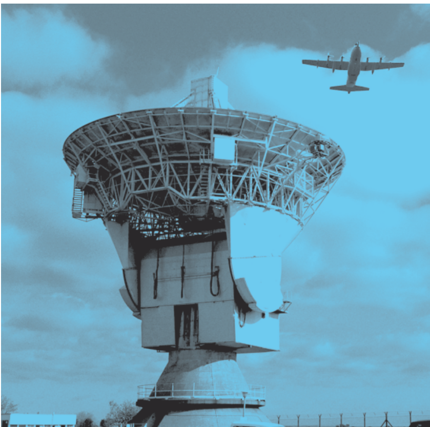
Figure 2. The UKMO-MRF Hercules C-130 flying over Chilbolton (UK), where all ground-based instruments were sited. CAMRa (3 GHz scanning radar), with its 25 m antenna, and Rabelais (35 GHz radar), with its small dish on the right-hand side of the large antenna, are also shown
