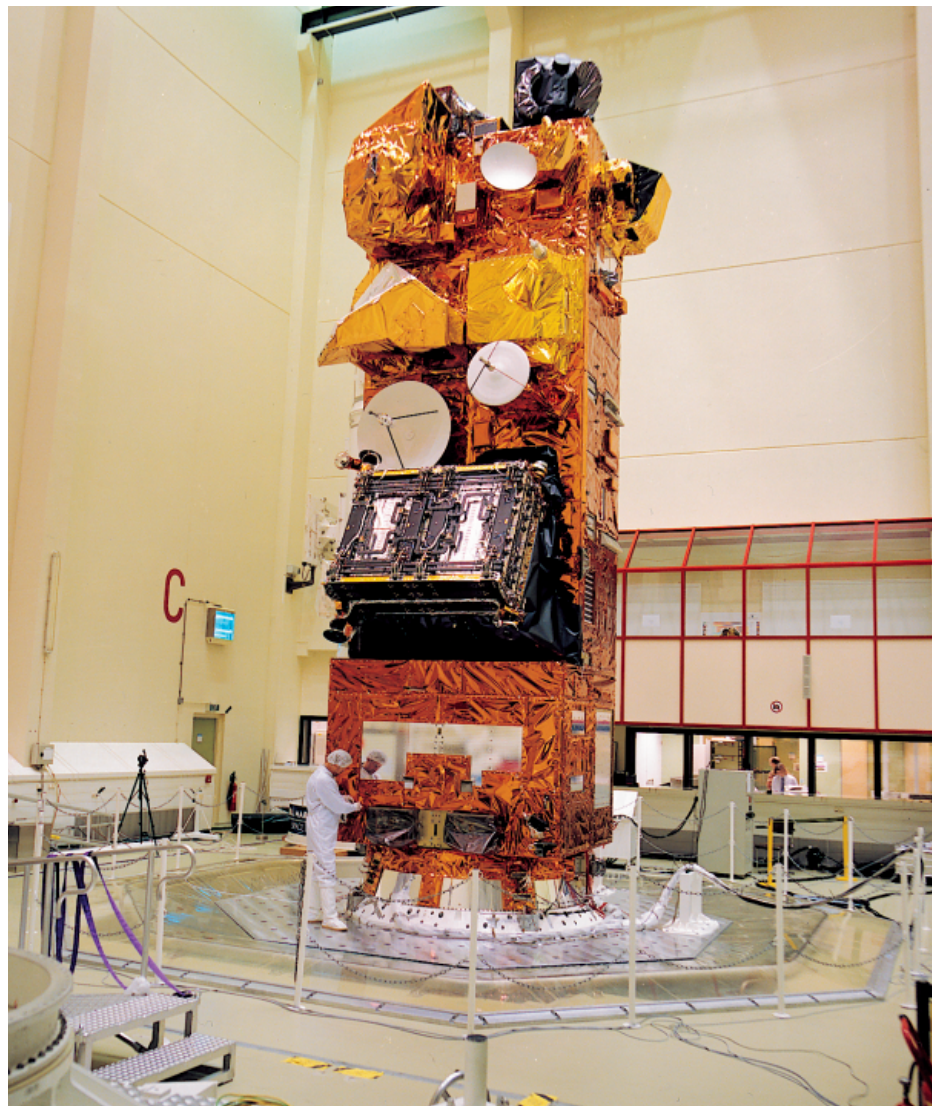
The Envisat flight-model satellite installed on the HYDRA test facility at ESTEC (NL)
