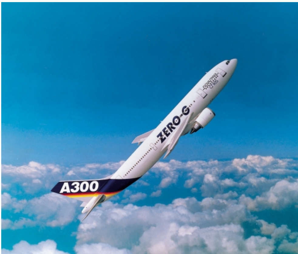
Figure 3. The A300 Zero-g during the injection phase before a parabola (courtesy of Novespace)
