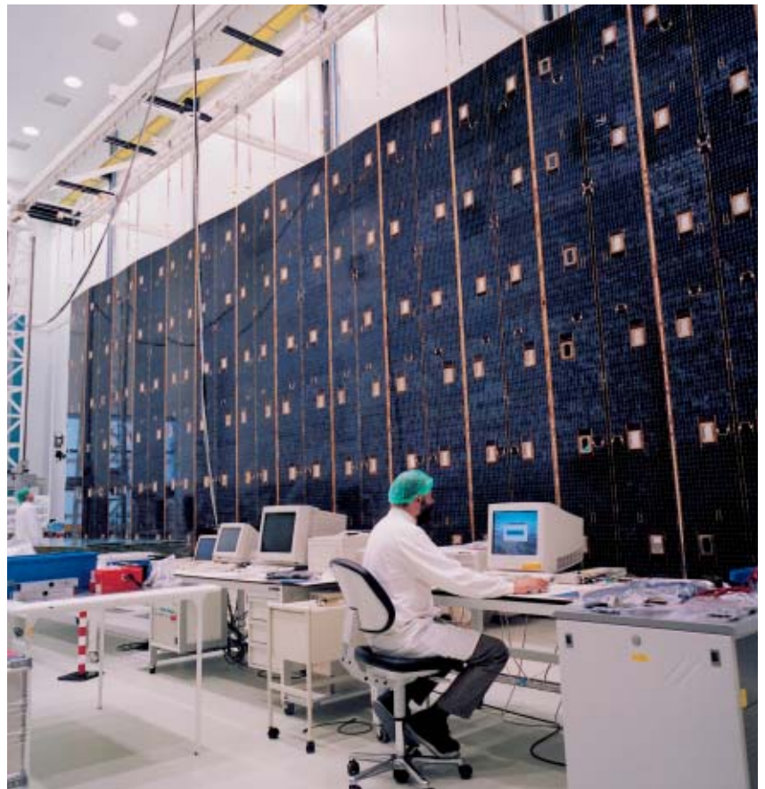
Figure 5. The solar array under test at Fokker (NL)
