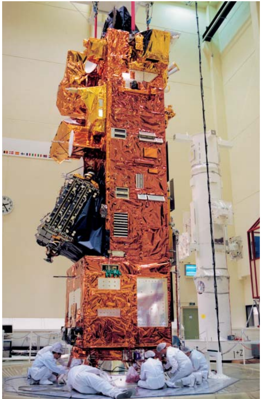
Figure 8. Envisat being installed on the HYDRA hydraulic shaker at ESTEC
