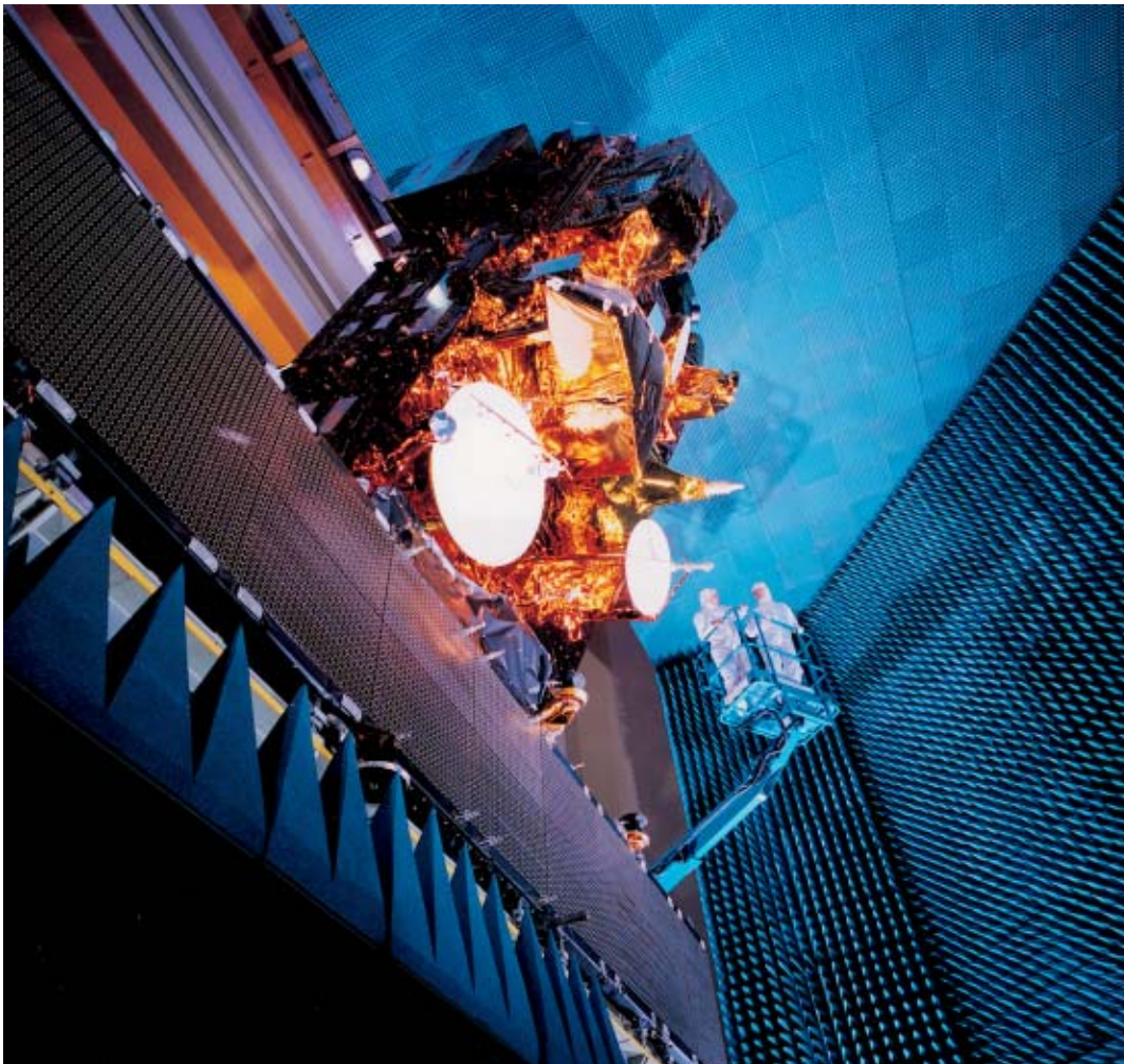
Figure 13. Flight model of Envisat being prepared for RF compatibility testing, with the ASAR antenna at the bottom of the picture
