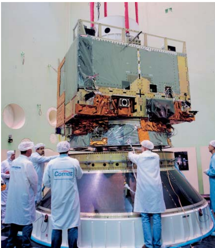
Figure 1. The Envisat Service Module being readied for shock testing in the ESTEC facilities
