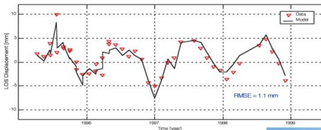
Figure 14. Measured line-of-sight displacement of the La Vilette Science Museum in Paris, compared to the modelled displacement due to temperature variations (courtesy of Politecnico di Milano, I)
