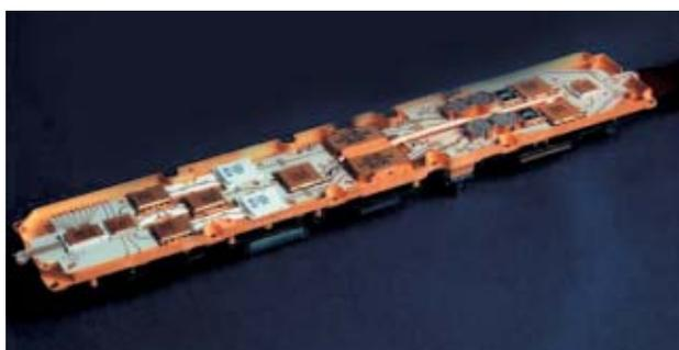
Figure 3. The ASAR transmit/receive module (courtesy of Alcatel, F)
