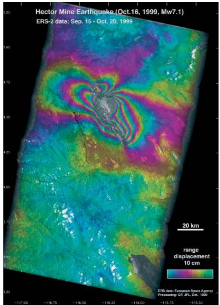
Figure 13. Interferometric map of the Hector Mine earthquake (1999) area in California showing the ground displacement along the radar line of sight. One full colour cycle represents 10 cm of range displacement (courtesy of JPL, USA)
