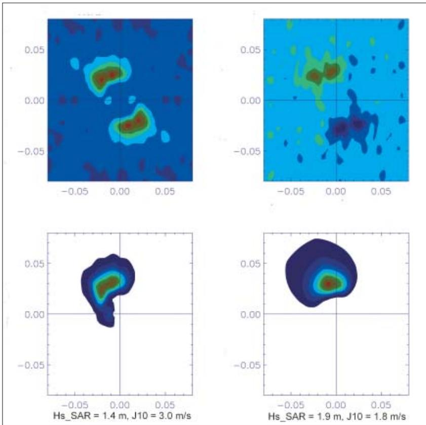
Figure 11. Real (top left) and imaginary (top right) parts of an image cross-spectrum (from ERS data), retrieved wave spectrum (lower left) and modelled spectrum (lower right) for comparison (Hs\_SAR = wave height, J10 = wind speed) (courtesy of NORUT, N)
