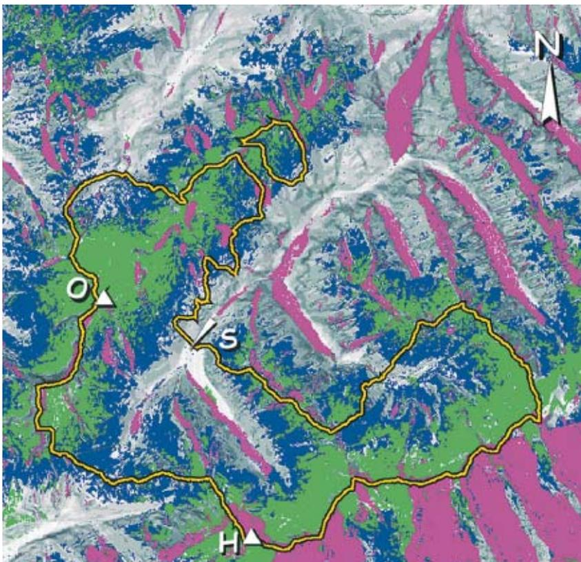
Figure 8. A snow map derived from ERS-2 ascending and descending passes over the Tyrolean Alps
