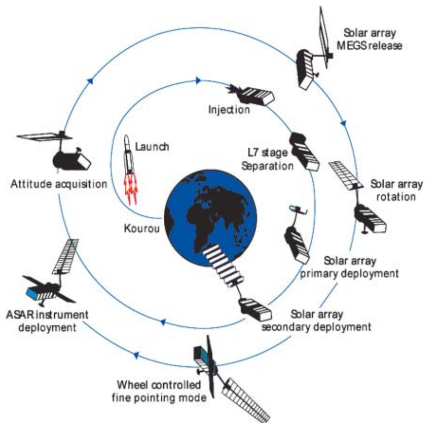
Figure 4. The Launch and Early Operations Phase (LEOP)
