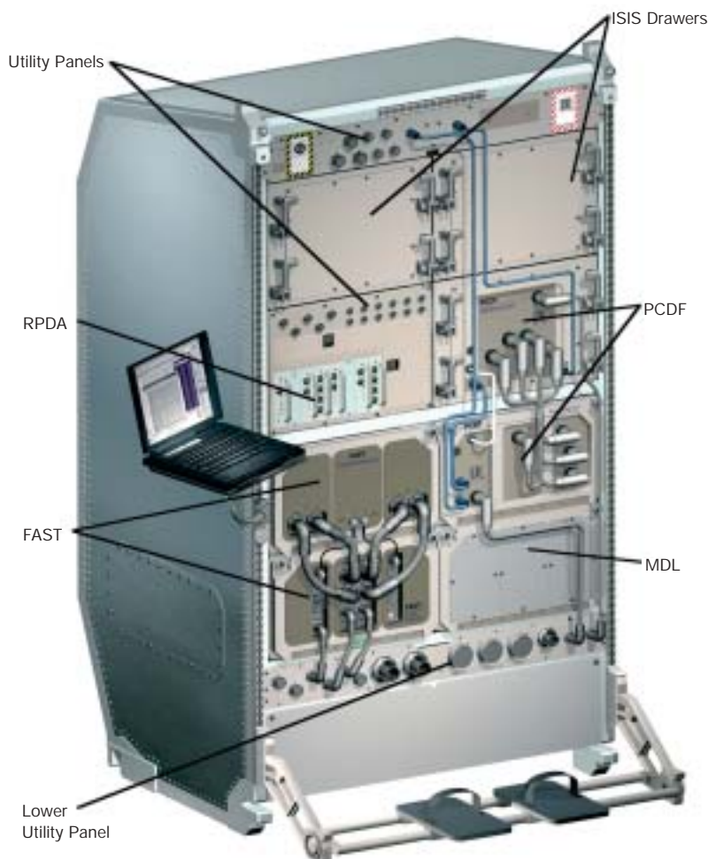
Figure 1a. Artist's impression of the EDR with two payloads (PCDF and FAST) integrated
