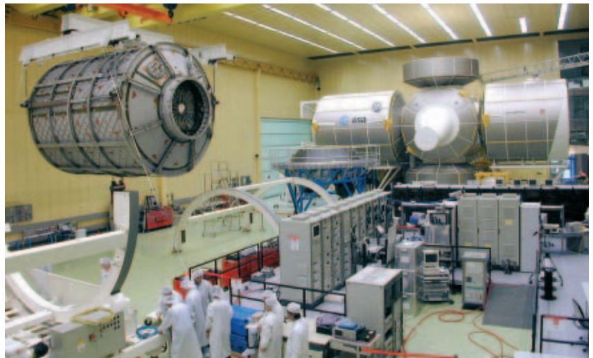
Figure 5. Columbus being moved to its integration stand in the prime contractor's integration hall. The ISS mock-up in the background includes Columbus and the Japanese Experiment Module, both attached to Node-2. The dark cabinets in front of the mock-up are the ETM racks, the lighter ones are the EGSE racks.
