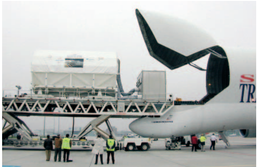
Figure 4. The Columbus flight unit being unloaded from its Beluga transporter at Bremen airport, on 27 September 2001. The servicer attached to the transport container provided atmospheric control.
