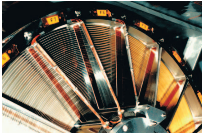
Figure 5. Close-up of an XMM-Newton Mirror Module. The 57 gold-coated thin nickel shells are concentrically stacked and fastened to spokes that help the shells maintain their correct positions. The nickel shells are about 1 mm thick, with a separation of about 4 mm between them
