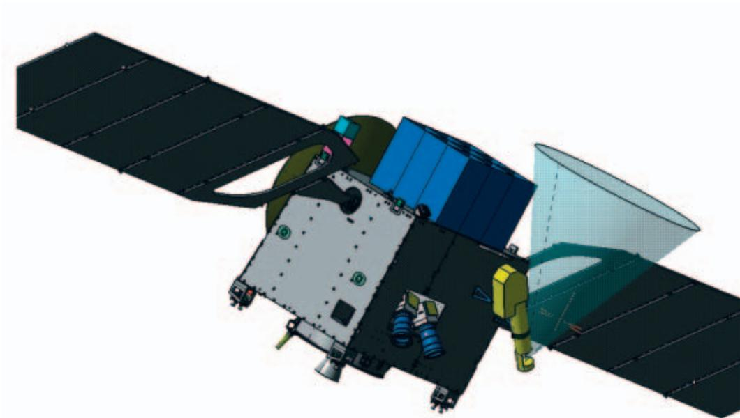
Figure 1. The Cosmic DUNE dust-telescope payload integrated on the Mars Express bus. The nine D2S modules form a telescope with a  $25^\circ$  half-width and a sensitive area of  $1 \text{ m}^2$ . ISIDE and CDA are attached to the impact plane of D2S, with each replacing one PVDF impact module (lower left). CIDA is attached to the side (optimum mounting angle  $40 \text{ deg}$ ), while PLASMON is mounted with a stand-off structure to measure the solar wind
