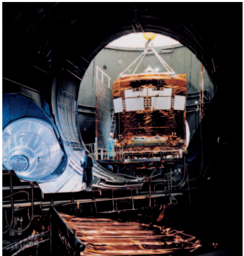
Figure 12. The ATV STM in ESTEC's LSS before thermal-balance testing
