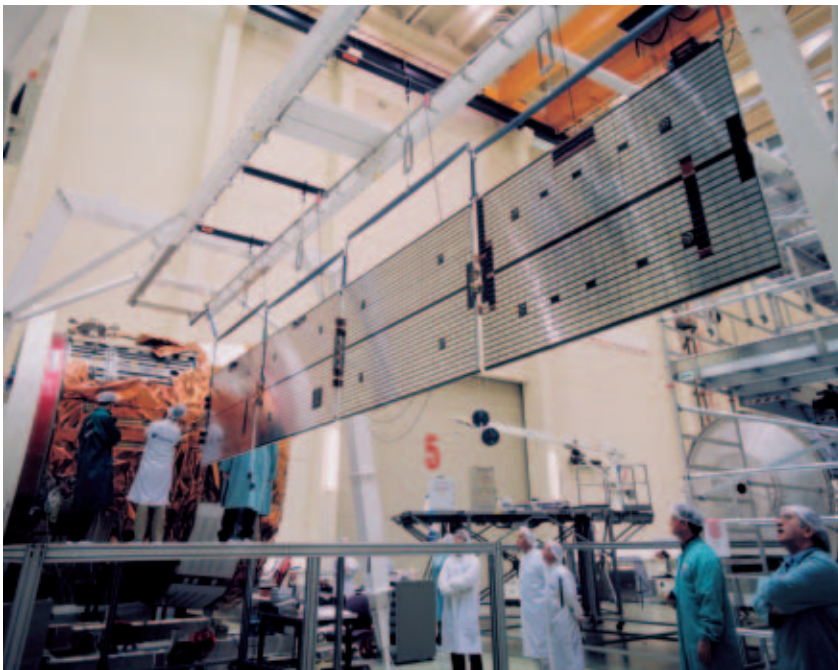
Figure 10. Solar wing under the deployment rig
