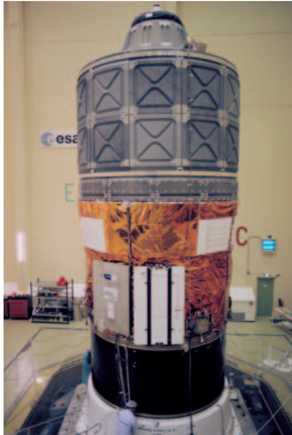
Figure 8. ATV (with SDM) modal tests on HYDRA
