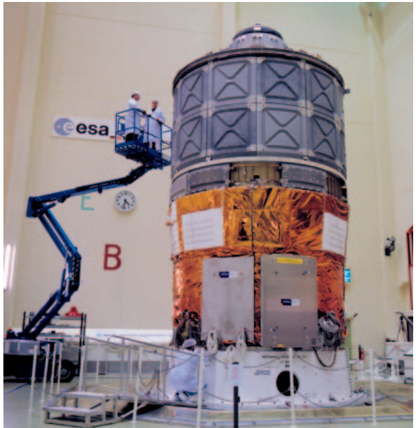
Figure 6. Longitudinal modal survey test set-up on HYDRA
