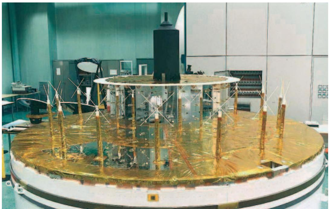
Figure 1. The flight-model MCP Antenna Subsystem
