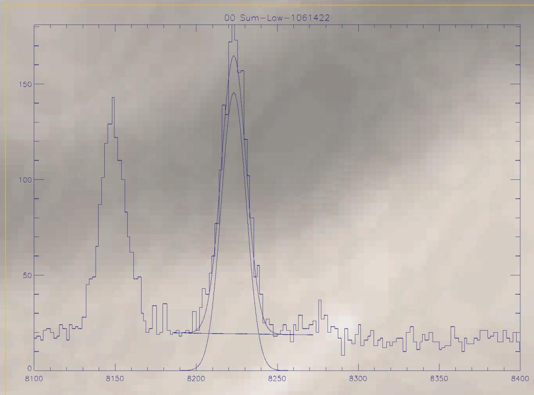
While looking to an empty space field, the Spectrometer sees spectral lines coming from its own germanium detectors (with the x-axis corresponding to the energy channels and the y-axis proportional to count rate). Here the two 69Ge lines at 1107 and 1117 keV can be clearly seen. The energy resolution around 2.5 keV indicates excellent instrument performance
