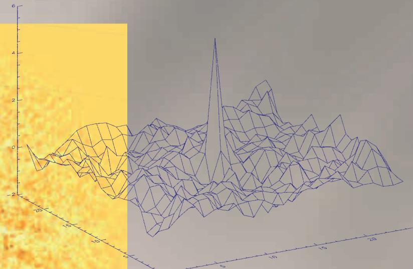
The first image of an X-ray star, Cen X-3, obtained with the Joint European Monitor for X-rays (JEM-X1) instrument. The 'star' is the small black dot near the centre. Although maybe unimpressive, the image gives the scientists confidence that the instruments are capable of detecting and accurately pinpointing X-ray sources in the sky. The contour plot (above) is based on data from the JEM-X2 instrument. (Courtesy of JEM-X Team)
