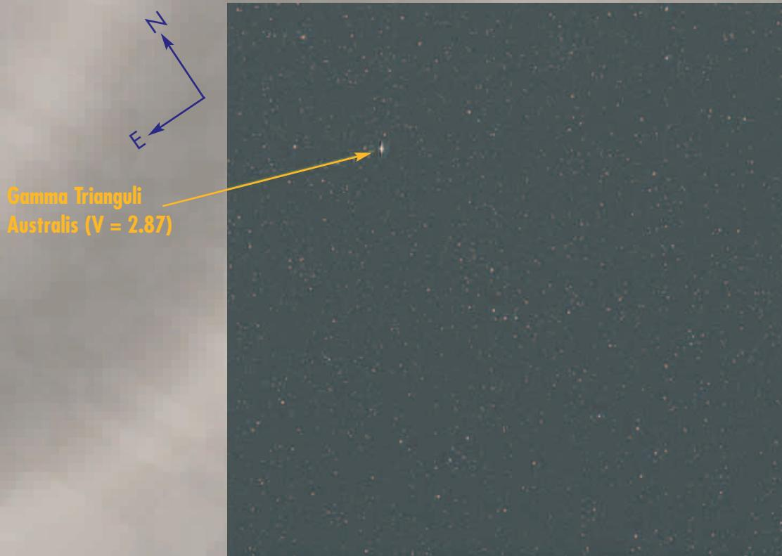
'First light' for Integral's Optical Monitoring Camera (OMC) just after the opening of its cover. The brightest star is Gamma Trianguli Australis. There is some saturation of the image pixels due to the combination of the brightness of the source and the relatively long integration time of ten seconds.
