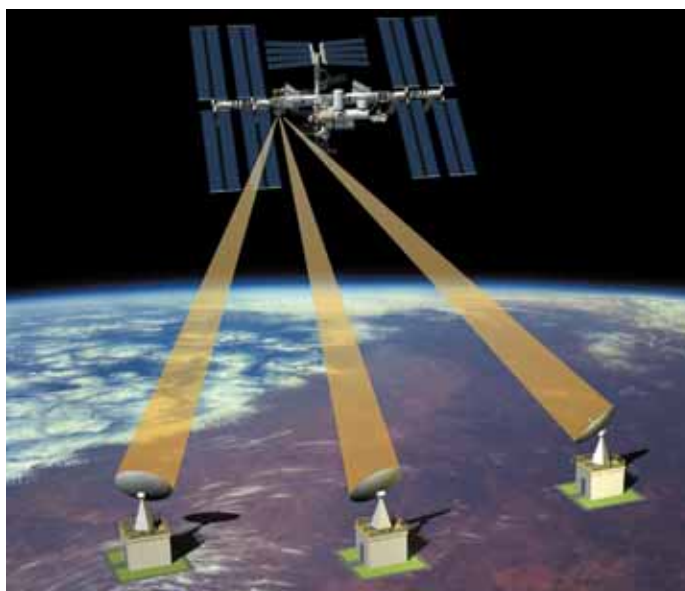
Research into cold-atom physics in space should lead to a factor 100 increase in atomic-clock frequency stability, with applications in fundamental physics, atmospheric physics and geodesy, navigation and telecommunications. This graphic shows the operational scenario for the Atomic Clock Ensemble in Space (ACES).
