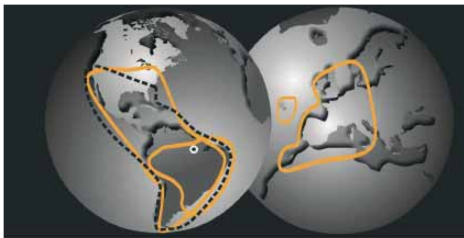
The coverages of the Amazonas satellite's three spot beams
