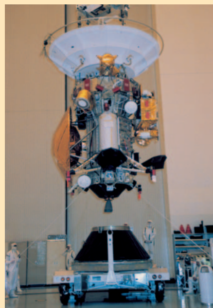
The Cassini spacecraft, with the Huygens probe mounted on the left side, being lowered onto its launch-vehicle adapter at Kennedy Space Centre (photo NASA)
