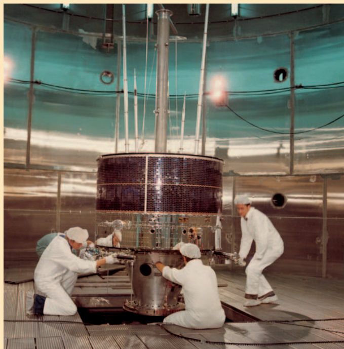
The GEOS spacecraft being prepared for boom-deployment tests in the Dynamic Test Chamber at ESTEC in Noordwijk (NL)
