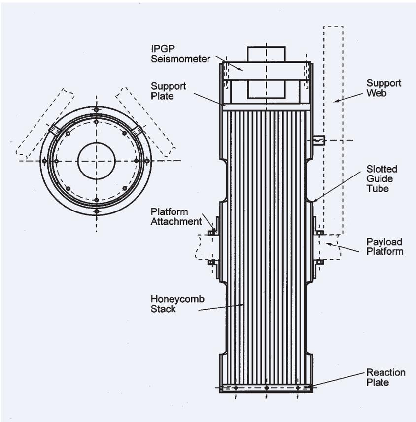
Figure 10. Guide-tube shock alleviation concept
