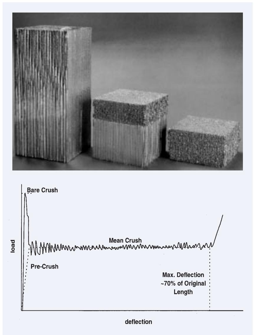
predictable manner. As shown in Figure 3, as the peak compressive load is overcome, crushing at a constant level is maintained until the material "blocks", forming a solid element. The area under the curve equates to the amount of energy that is dissipated. The manufacturers quote honeycomb crushing strengths only for static crushing and we therefore included dynamic tests in our study.
