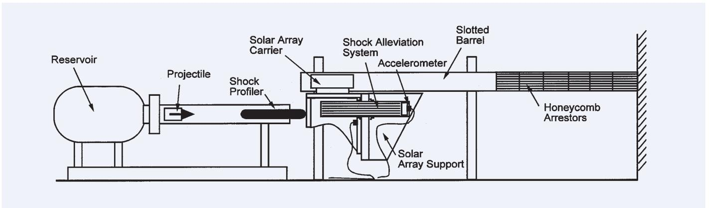
Figure 12. The revised test configuration
