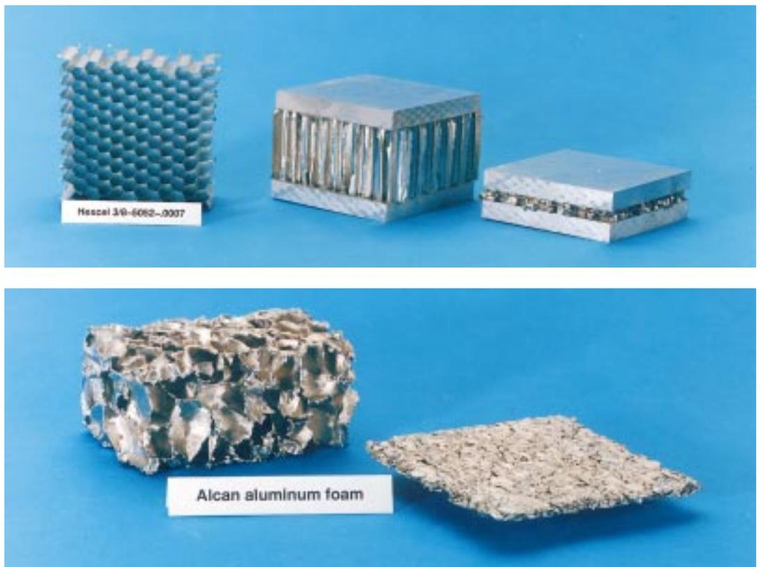
Figure 8. Aluminium honeycombs and foams tested for shock absorption
