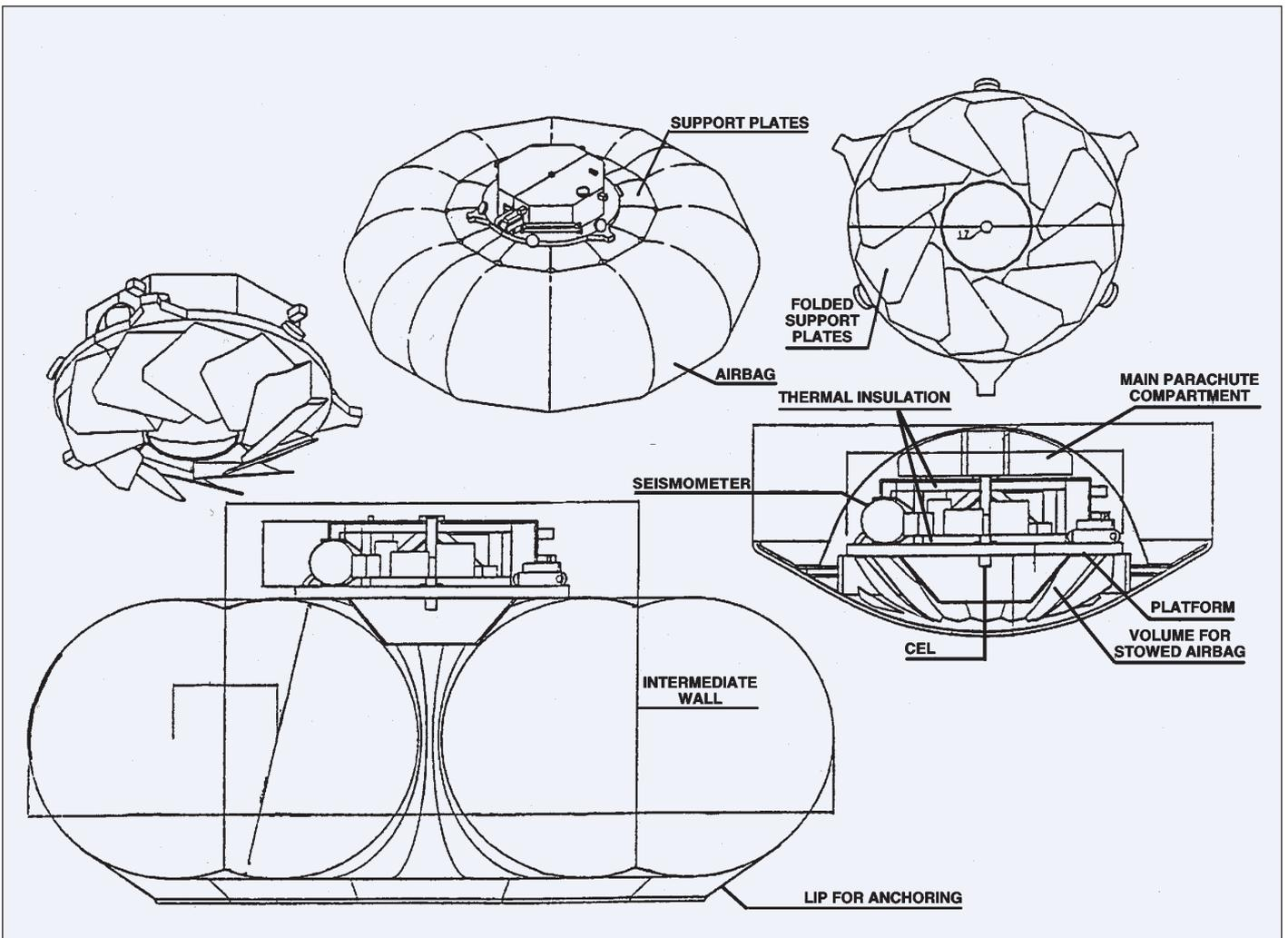
requirements. These semi-hard landers do not penetrate the planetary or cometary surface.
