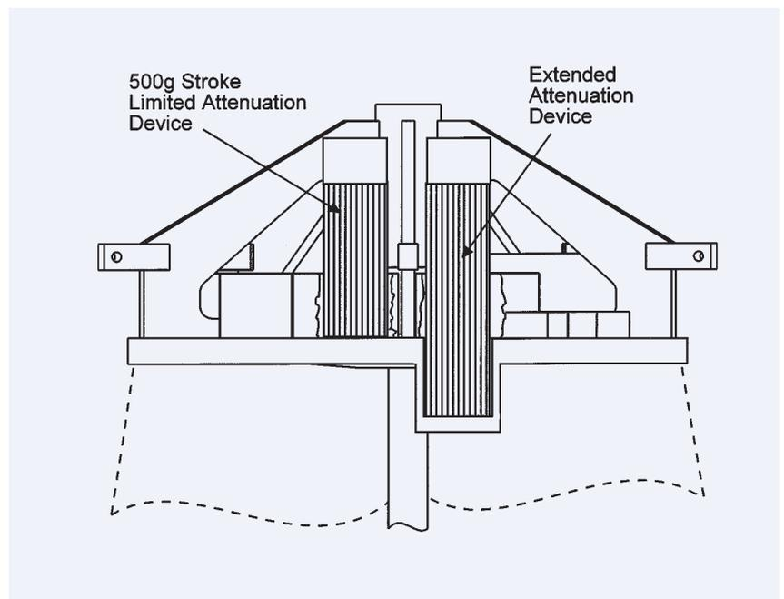
Figure 6. Incorporation of extended attenuation device
