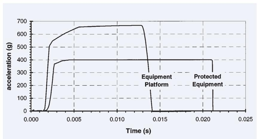
Figure 7. Acceleration profiles of platform and protected equipment
