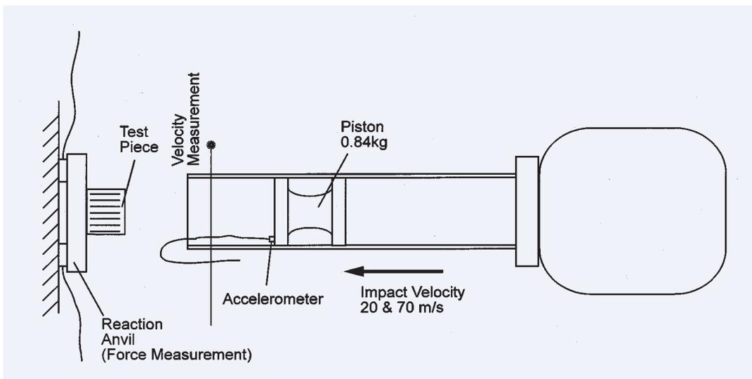
Figure 9. Air-gun facility used for dynamic crushing tests
