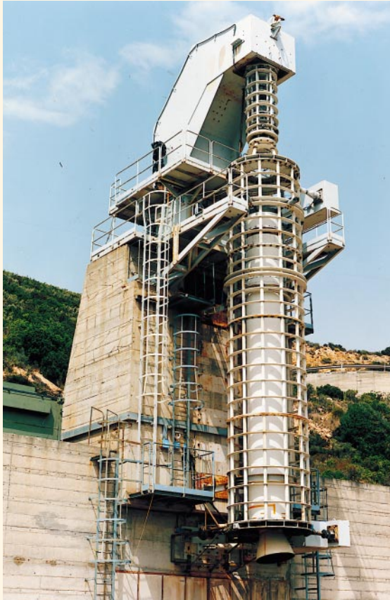
Figure 3. Ariane-4 strap-on-booster test stand in Sardinia (Italy), and a full-scale firing test sequence in 1997 to qualify a new ingredient in the solid propellant's composition © A. Constanzo for ESA/CNES/Arianespace
