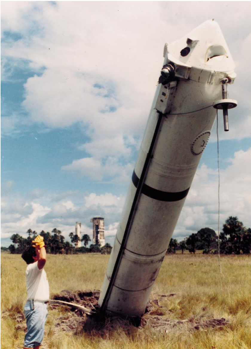
Figure 2. Post-flight inspection of Ariane-4 solid boosters at the Guiana Space Centre provides important information that cannot be communicated by telemetry alone: behaviours of thermal protection, nozzles, fields joints, etc. © ESA/CNES/Arianespace
