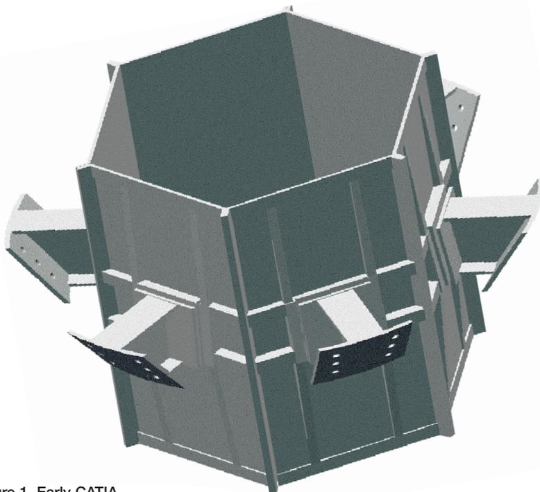
Figure 1. Early CATIA concept model of a cone-mounted option for the TEAMSAT box
