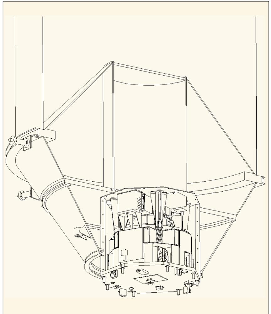
Figure 3. Cutaway view (CATIA model) of TEAMSAT mounted in Maqsat-H, including TEAMSAT cone-mounted sensors
