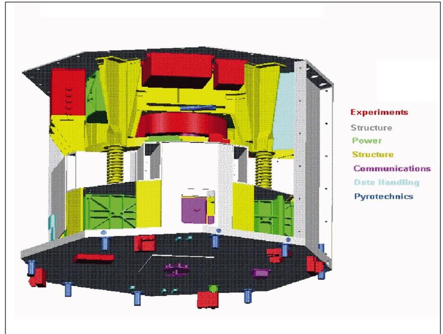
Figure 2. Final CATIA Master Model of the TEAMSAT system, colour coded to identify sub-system groups
