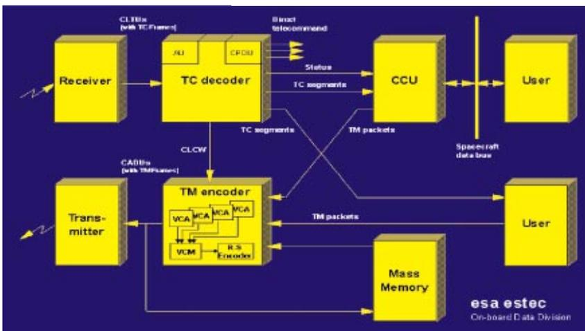
Figure 9. A typical onboard telemetry and telecommand data-processing approach for an ESA spacecraft
