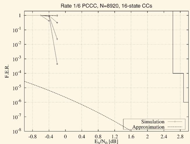
Figure 8. Simulated FER versus  $E_b/N_0$  curves for 16-state rate 1/6 turbo code and spread interleaver ( $N=8920$ )
