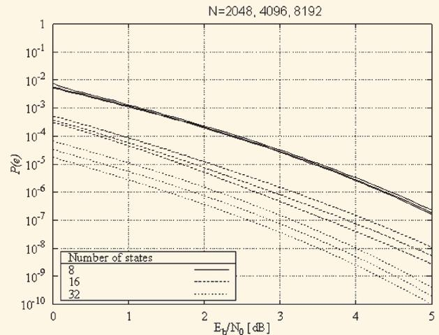
Figure 6. FER versus  $E_b/N_0$  bounds for proposed rate 1/2 turbo codes
