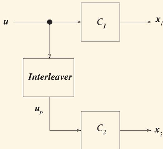
Figure 5. The turbo-encoding concept
