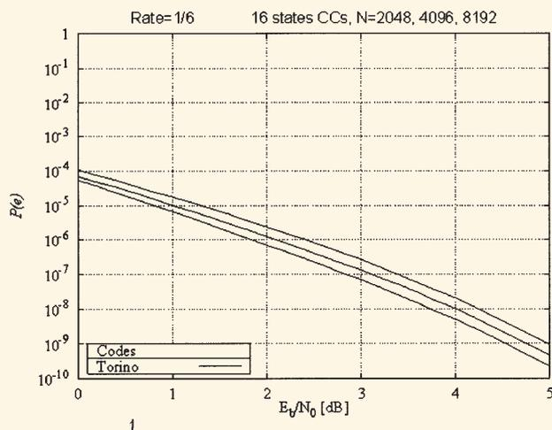
Figure 7. FER versus  $E_b/N_0$  bounds for 16-state rate 1/6 turbo code
