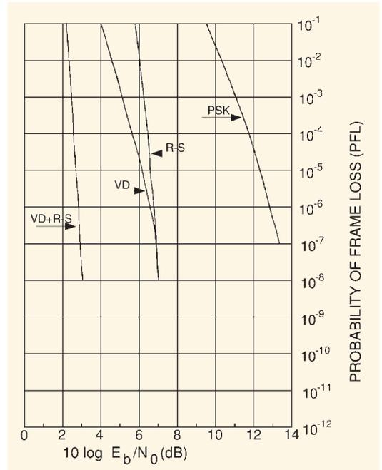
Figure 4. Frame Error Rate (FER) performances of the various CCSDS codes
