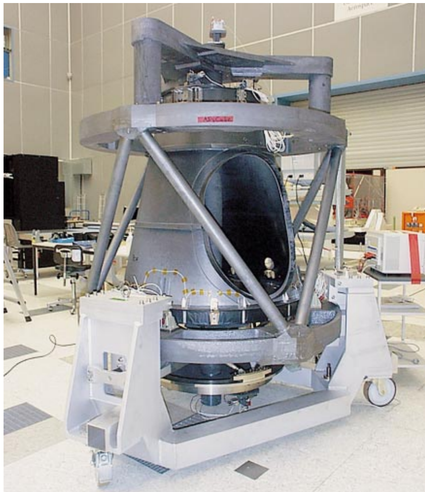
Figure 9. Large verification structure for the SEVIRI thermal-stability test; the monolithic ceramic structure is 150 cm in diameter and 200 cm high
