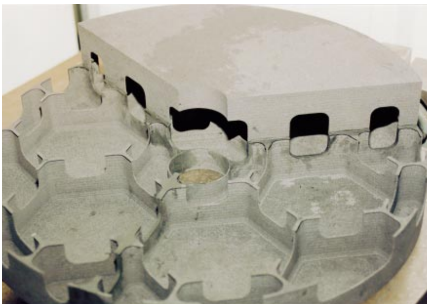
Figure 5. Lightweight closed-back structure with a diameter of 45 cm, made from six pieces joined in the green-body state and infiltrated to a single unit
