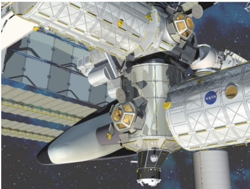
Figure 5. ESA is providing the Station with two Cupolas and, in a separate agreement with NASA in part return for launching Columbus aboard the Space Shuttle, Node-3, seen here in the centre of the illustration. The Crew Rescue Vehicle, at left, may become part of a later arrangement between ESA and NASA (ESA / D. Ducros)
