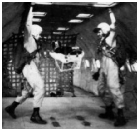
An early parabolic-flight cardiology experiment onboard NASA's KC-135 aircraft in which a free-floating bed was used to record a ballistocardiogram for the test subject and measure the expulsion of blood from the heart into the bodily circulation under different g-forces (photo NASA)
