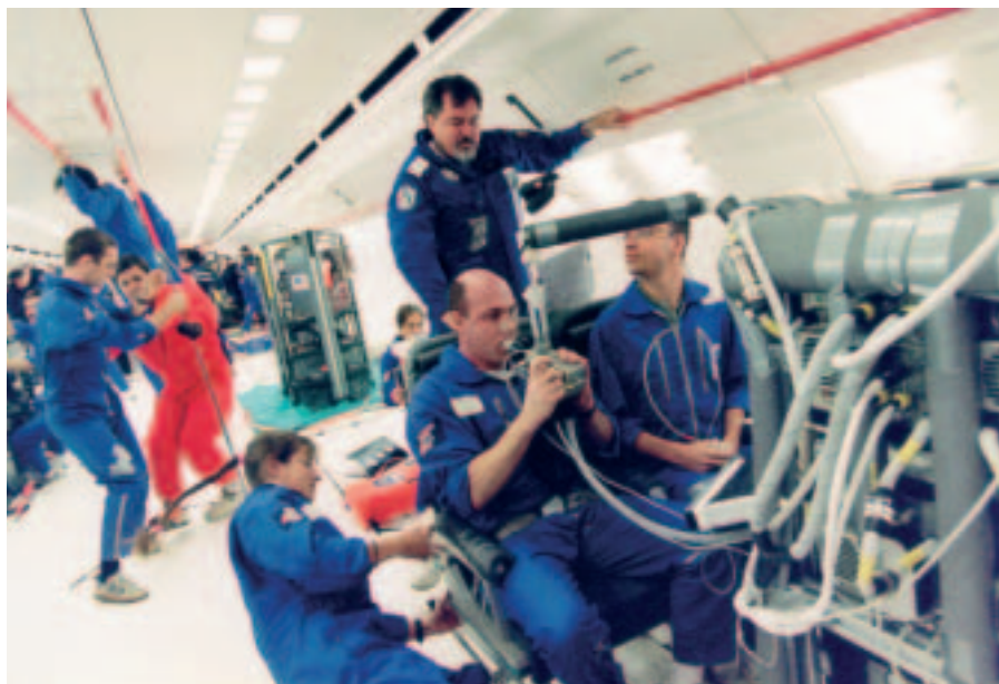
The ARMS equipment was used onboard the Airbus A300 'Zero-G' for several respiratory experiments in 1999. Here Prof. G.K. Prisk (Univ. California, San Diego, USA) is monitoring ESA astronaut Andre Kuipers acting as the test subject
