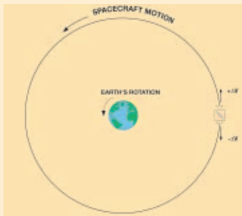
The geostationary orbit and the concept of tangential and out-of-plane burns
