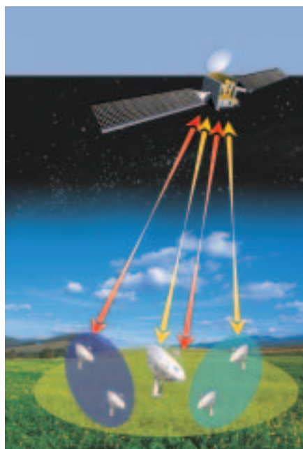
AmerHis provides connectivity between spot-beam coverage areas without the need for double hops between ground and spacecraft
