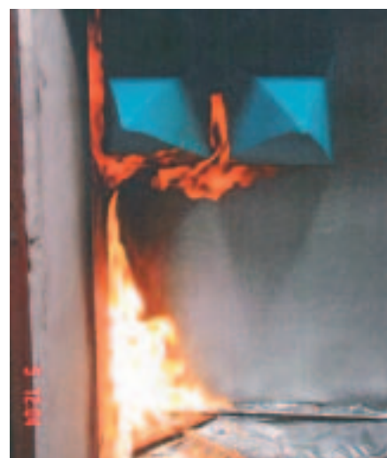
Fire-resistance testing of the carbon-loaded foam pyramids at TNO in Delft (NL)
