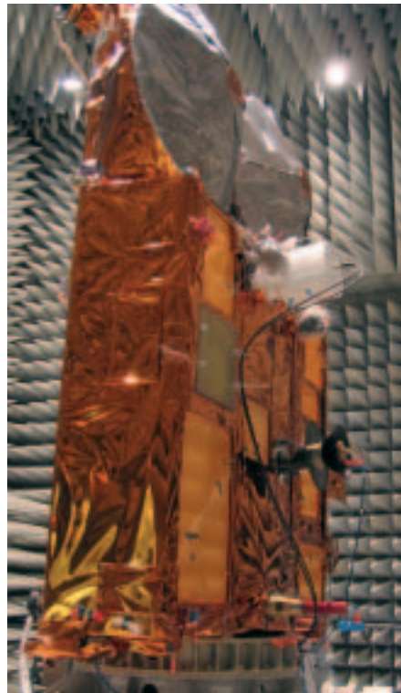
CryoSat in the EMC chamber at ESTEC in Noordwijk
