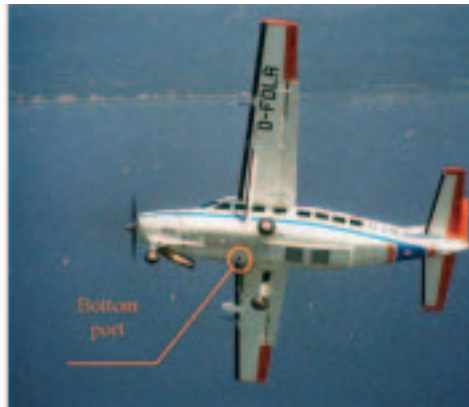
The SmartScan airborne flight-test configuration
