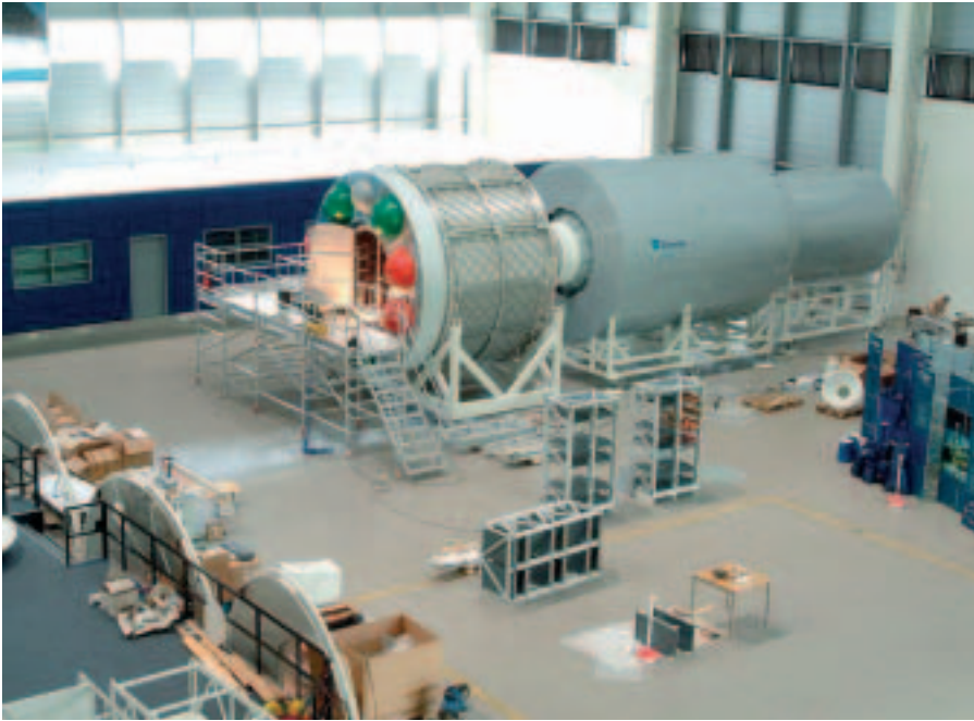
The EAC Training Hall, with the ATV simulator under construction
