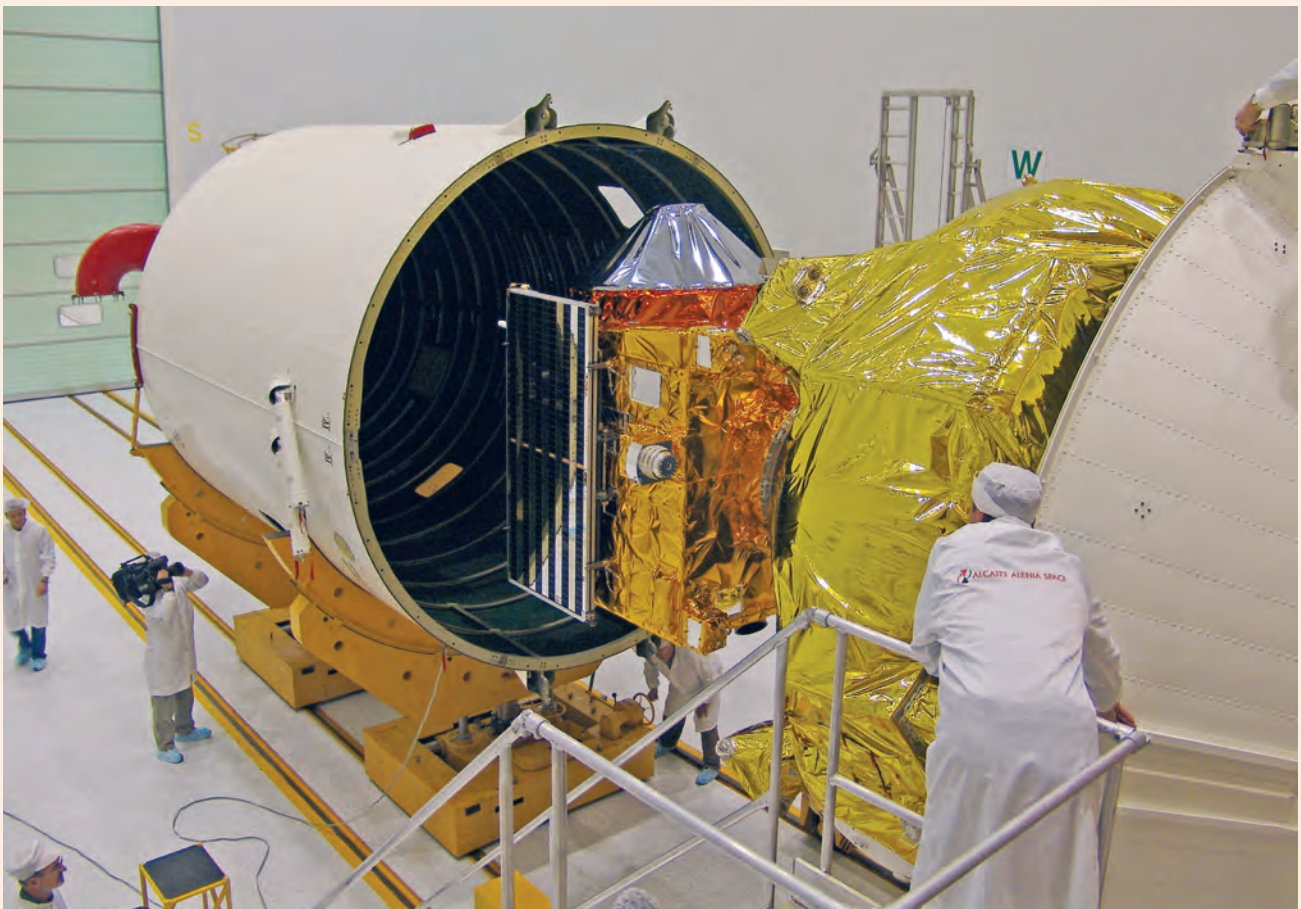
The Soyuz fairing being moved over the horizontally tilted stack of the Venus Express spacecraft and the Fregat upper stage
