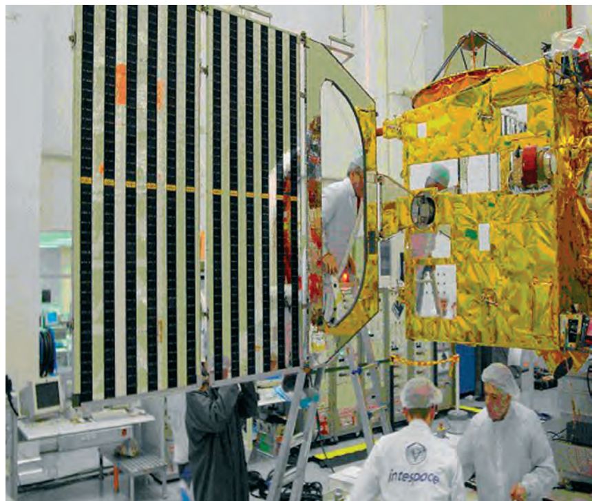
One of the solar-array wings after a successful deployment test at Intespace in Toulouse (F)
