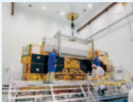
The solar array is attached to MetOp during final reassembly at Baikonur
