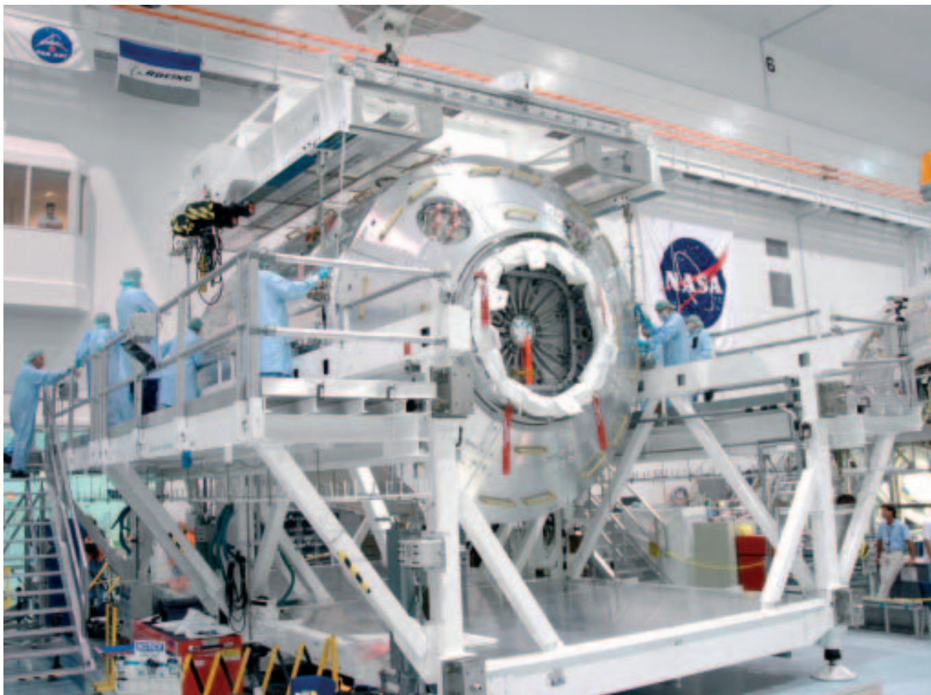
Columbus is installed in its processing stand. Almost hidden at far right is Node-2, which Columbus will be attached to on the ISS
